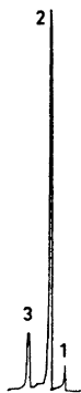
Fig. 1. Gas chromatogram of DETA. Temperature of analysis 250°C, for other conditions see experimental part. Formulas and mass spectra of fractions are given in Tables 1 and 2. Fraction 1 consists of an unresolved mixture.
